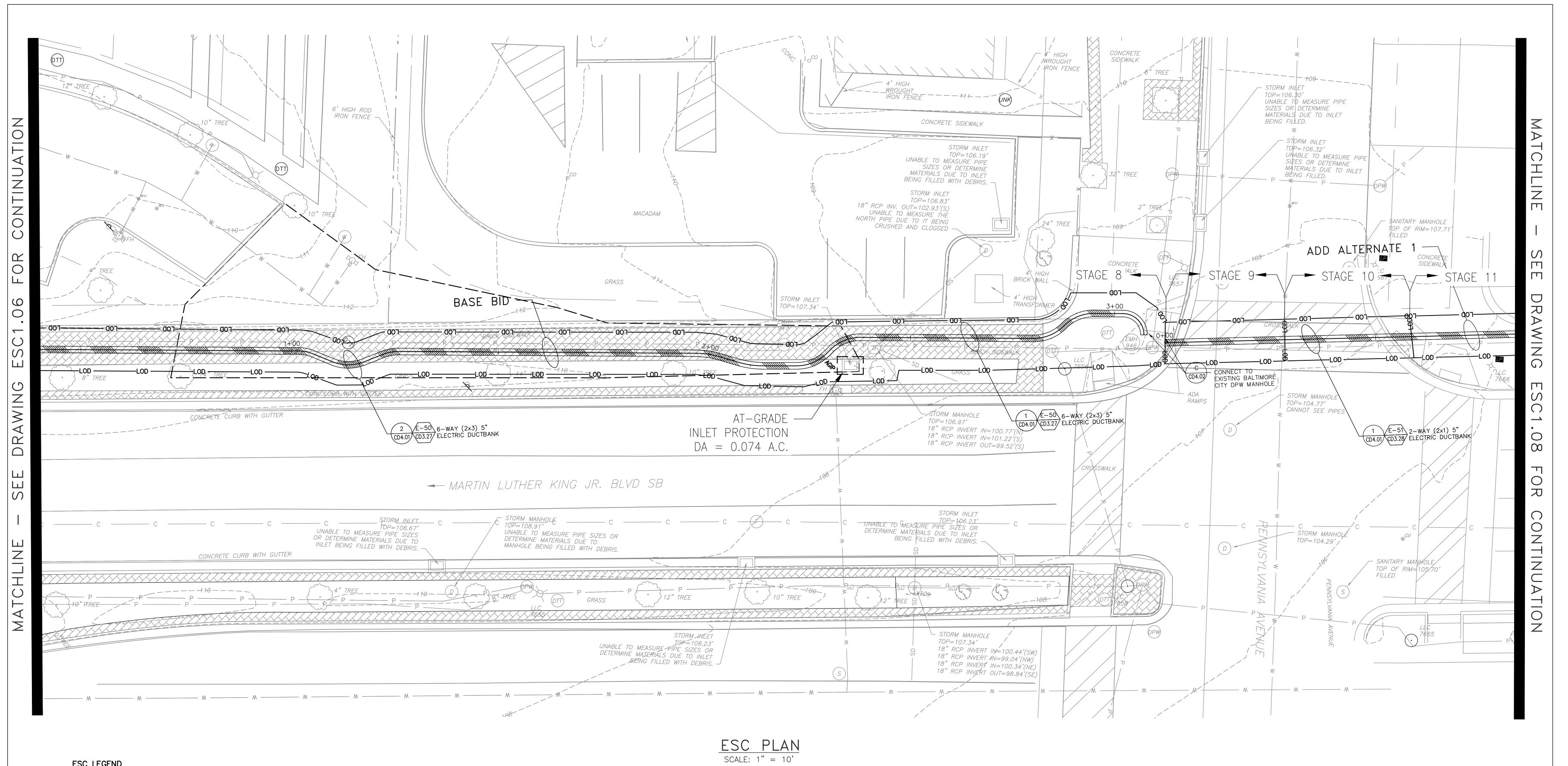
ESC LEGEND — LOD — LIMIT OF DISTURBANCE — — DRAINAGE AREA COMBINATION **INLET PROTECTION** CURB INLET PROTECTION AGIP AT-GRADE INLET
