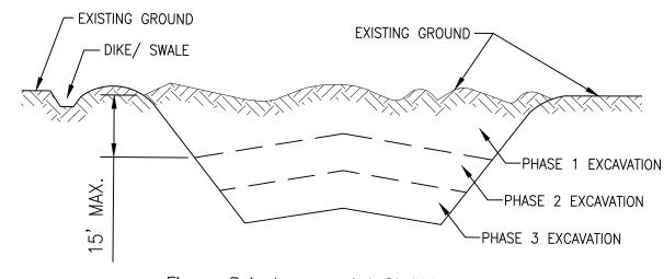
Figure B.1: Incremental Stabilization — Cut
